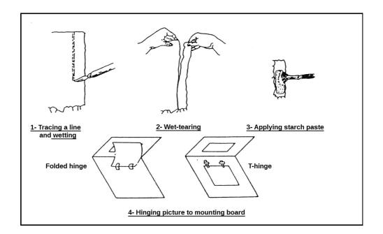
The Japanese paper is cut by tearing it along a line moistened with water. The print is then centered under the window and secured with paper hinges and starch glue.
