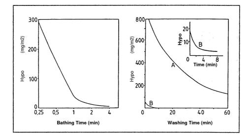
The figure above shows the effect of softening a sheet film in a sodium sulfite solution after fixing (left). After two minutes of soaking, the film was washed (curve B right) and the result compared to a prolonged water wash (curve A right) without wash-aid.
