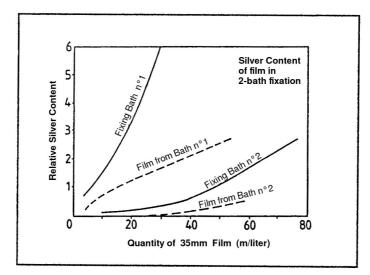
G. Eaton<sup>20</sup> shows in the graph above that most of the silver is dissolved in the first bath, and that the fixing is then completed in a second fresh bath where the silver concentration remains very low. The dashed lines show the silver retention in the processed film. A similar phenomenon also occurs with paper emulsions.
