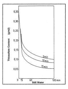
The papers of the test were rinsed respectively in water flowing at 4 l/min for 5, 10 and 15 minutes. This in the first compartment of the Deville vertical washer. After that, the water supply was cut off and the rack with the papers was transferred to the second washing compartment. The papers soaked in pure water for periods of up to 180 minutes. These papers were tested at regular intervals to obtain the wash curves shown above.
