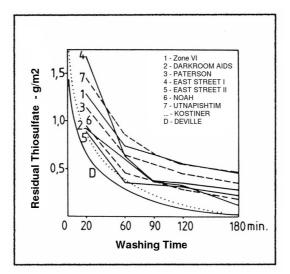
The washing curve of the recently discontinued Kostiner washer was added in dashed lines, as well as a "D" curve for the French Deville washer. The washing scheme of all these tests is almost identical, so that the results can be compared to each other.
