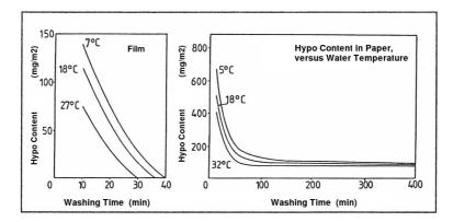
Eaton<sup>28</sup> mentions that it is desirable to maintain the temperature of the wash water between 14 and 17°C. The effect of temperature on the washing time for film and baryta emulsions is presented above. Once again, this chart makes clear that it is easy to achieve complete elimination for films, but impossible for paper.
