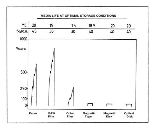
Compared to the most modern substrates, black and white emulsions processed and stored under optimal conditions remain the most stable.
