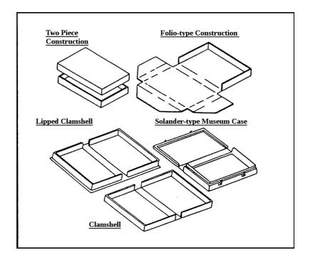
Archival boxes designed for long-term preservation are made exclusively of acid-free materials. These sometimes less luxurious boxes can be made of acid-free corrugated cardboard: they are then designed to be assembled by folding, without metal staples.
