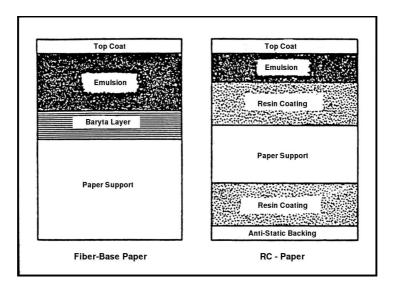
A modern variant is Resin Coated (RC) paper. Here, the paper support is covered on both sides with a layer of polyethylene (PE paper). The advantages of resin coated paper are as follows:<sup>7</sup>
