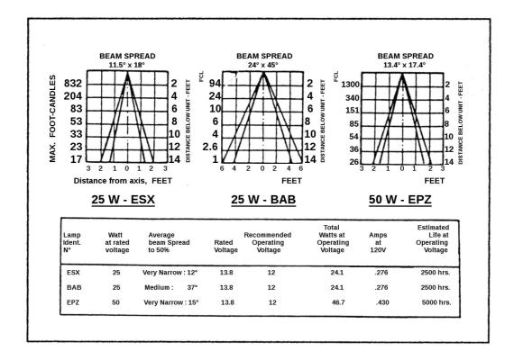
Low voltage halogen lamps can have different lighting angles, which makes it possible to adapt them to a wide variety of exhibition conditions.
