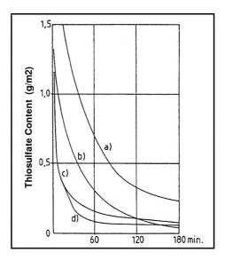
Curve d), corresponding to 15 minutes of washing in running water, combined with the rapid fixing curve, shows how the soaking of the second wash phase improves the final wash without additional water consumption.
