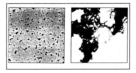
Small silver particles give warm tones (leaning towards yellow, red and brown), while relatively large silver particles produce more neutral black tones. The shape of the silver particles is also important. The stretched or irregularly shaped silver particles make the image more neutral than the same amount of spherical particles.
