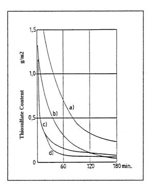
**Curve a** corresponds to the fixing salts elimination by a running water wash after a 2-bath fix in Agefix 1+9, without wash-aid after fixing.
