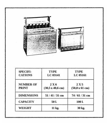
The washing compartment has a removable rack for the prints to be washed. The latter are held by nylon threads and can not stick together. The water supply is through the bottom of the washer and the fixing salts are removed by the water flow under the rack. A series of tests were carried out with the Deville washer, in order to develop an efficient washing method while saving water. This study was carried out with the following material:
