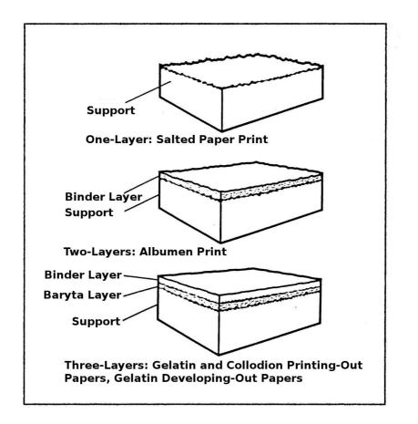
A single layer structure where the print is simply composed of a paper substrate on which the photosensitive solution is applied. The latter penetrates into the fibers of the paper; the image appearing after processing will be totally matte.
