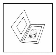
The mounting board described above forms the back of the assembly. The front of the latter is usually composed of a thicker acid-free cardboard with a beveled window cut to the dimensions of the print. The two boards are joined from the inside, along the longest dimension, by a hinge tape.
