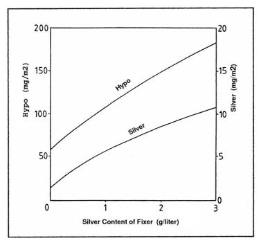
Above, a graph showing the silver and thiosulfate content of a silver print as a function of the fixer's silver content. A stop bath was used to keep the acidity of the fixer constant. Here, a single weight Kodak Velox paper was fixed in the Kodak F-5 fixer for 10 minutes, then rinsed for 30 minutes.
