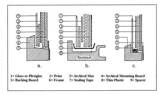
Fig. (a) shows the traditional method in which a sandwich consisting of the print (2) and the conservation mounting with its mat (3) and its mounting board (4) is clamped between a glass or plexiglass plate (1) and the backing of the frame (5), the latter being sealed all around (7) to prevent the penetration of dust.
