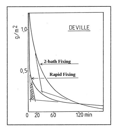
The washing curves obtained made it possible to estimate the duration of washing phase 1, i.e. the required washing in running water. This is:
