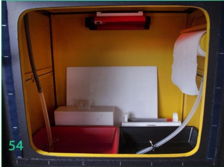
The second door gives access to an opening large enough to pass my shoulders. It is equipped with a sleeve made from yellow opaque fabric, fixed with Velcro strips on one side and provided with a rubber band on the other.
