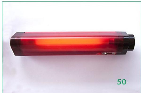
When there is not enough light outside to use the window, a battery-powered fluorescent tube, provided with the same filters, can be used instead. See picture 50.
