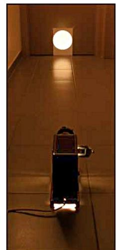
I put a black pvc sheet with a 10mm hole (checked with a micrometer) in a slide mount. This mount is then put in the projector which is aimed at a sheet of drawing paper fixed on a vertical support. This allows me to draw the precise diameter of the projected circle, and finally the circle itself. I part the diameter in 10 divisions, and each of them in 10 subdivisions (*see above*).
