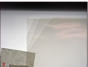
To register the negatives, I mounted a matte glass in a system similar to a painter's easel. I place it in front of a window so that the light illuminates the glass from behind.
